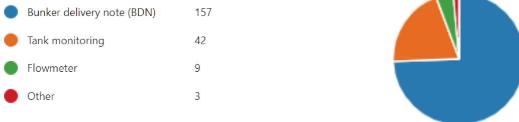
Figure 2: Number of ships adopting the various methods for collecting fuel oil consumption data
